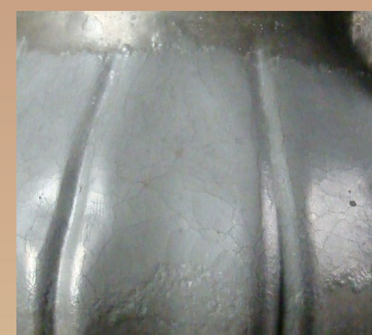
Detail of fragmentary surface coating on the base metal. (right)
